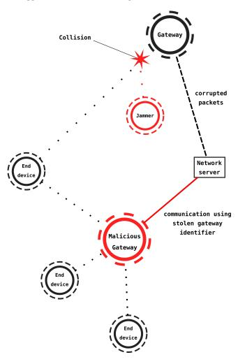
Figure 6: impersonation attack using jamming
