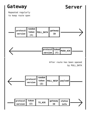
Figure 4: Packet Forwarder Protocol downlink sequence diagram
