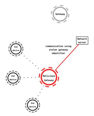
Figure 5: impersonation attack disconnecting the gateway
