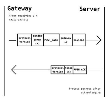
Figure 3: Packet Forwarder Protocol uplink sequence diagram
