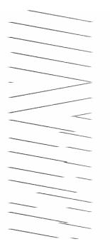
Figure 2: Spectrogram excerpt of a LoRa chirp y-axis: Time, x-axis: Frequency | taken from [5]
